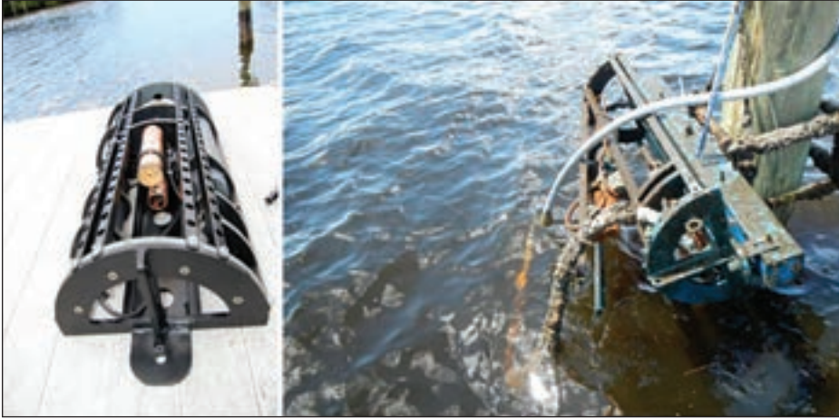
At left, the new RECON sensor before installation. At right, the sensor at Beautiful Island after a lightning strike. The boards were fried, there were burn marks and the rail holding the sensor on has been flown off.
